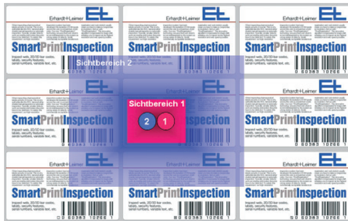
Figure 3: Dual camera principle with different fields of view.
